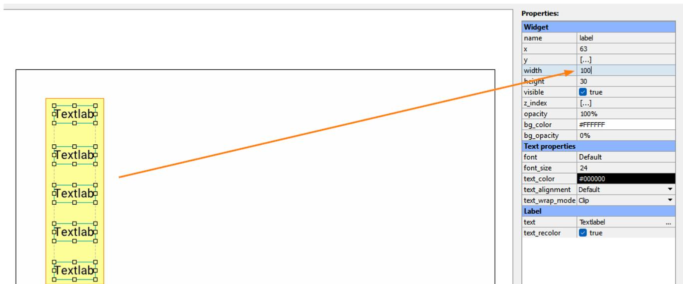
The screenshot shows a GUI editor interface. On the left, a vertical column of five 'Textlab' widgets is selected, indicated by a yellow dashed border. On the right, the 'Properties' panel is open, showing a list of properties for the selected widgets. The 'width' property is highlighted in blue, and an orange arrow points from it to the selected widgets. The 'Properties' panel is structured as follows:
