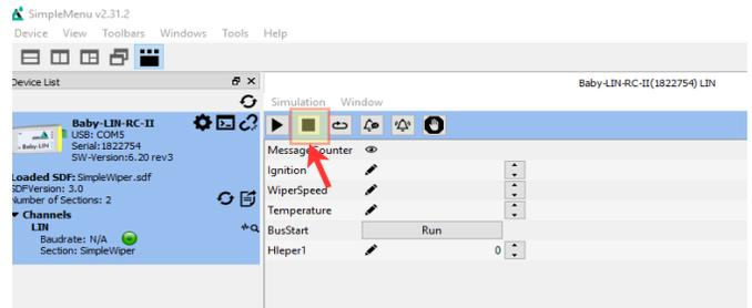
Step 3: Load SDF into Baby-LIN
