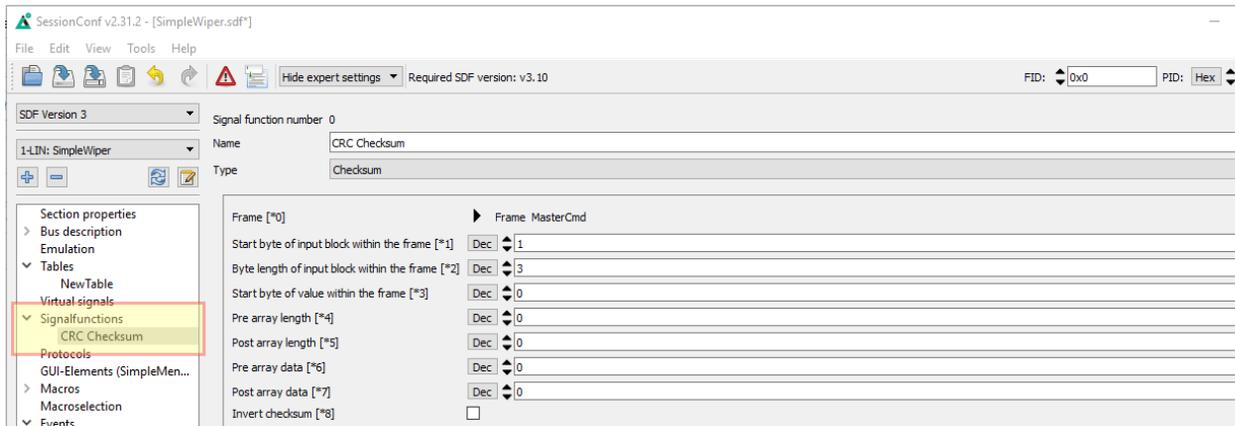
The parameters \*4 to \*7 define an optional prepend and postpend buffer with up to 8 byte values, which are then prepended or appended to the data of the real frame before the calculation.
