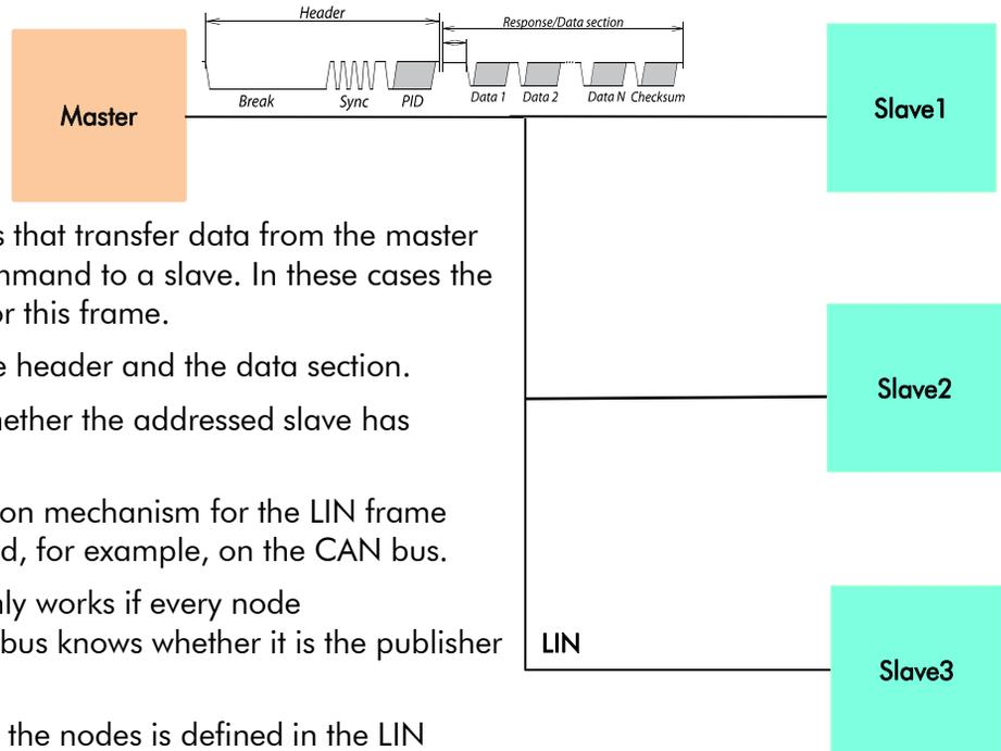
Of course, there are also frames that transfer data from the master to a slave, e.g. to transmit a command to a slave. In these cases the master is defined as publisher for this frame.
