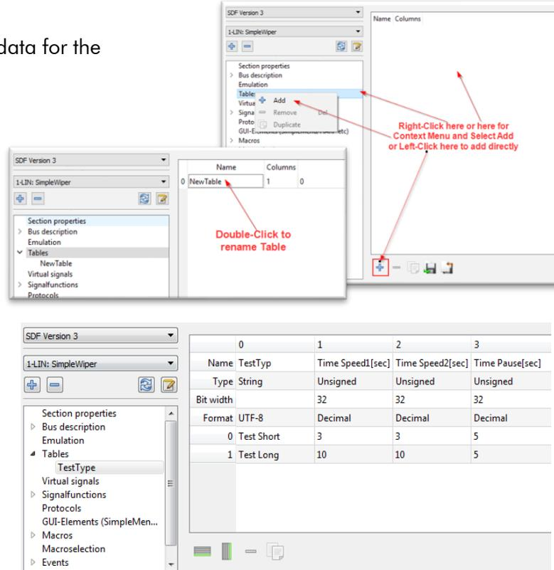
Here the completed example table with 5 test variants, column 0 contains the name of the test, columns 1...3 define certain time specifications for the individual test variants.
