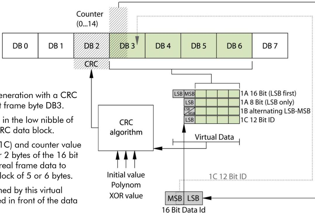
Example of a CRC generation with a CRC data block starting at frame byte DB3.
