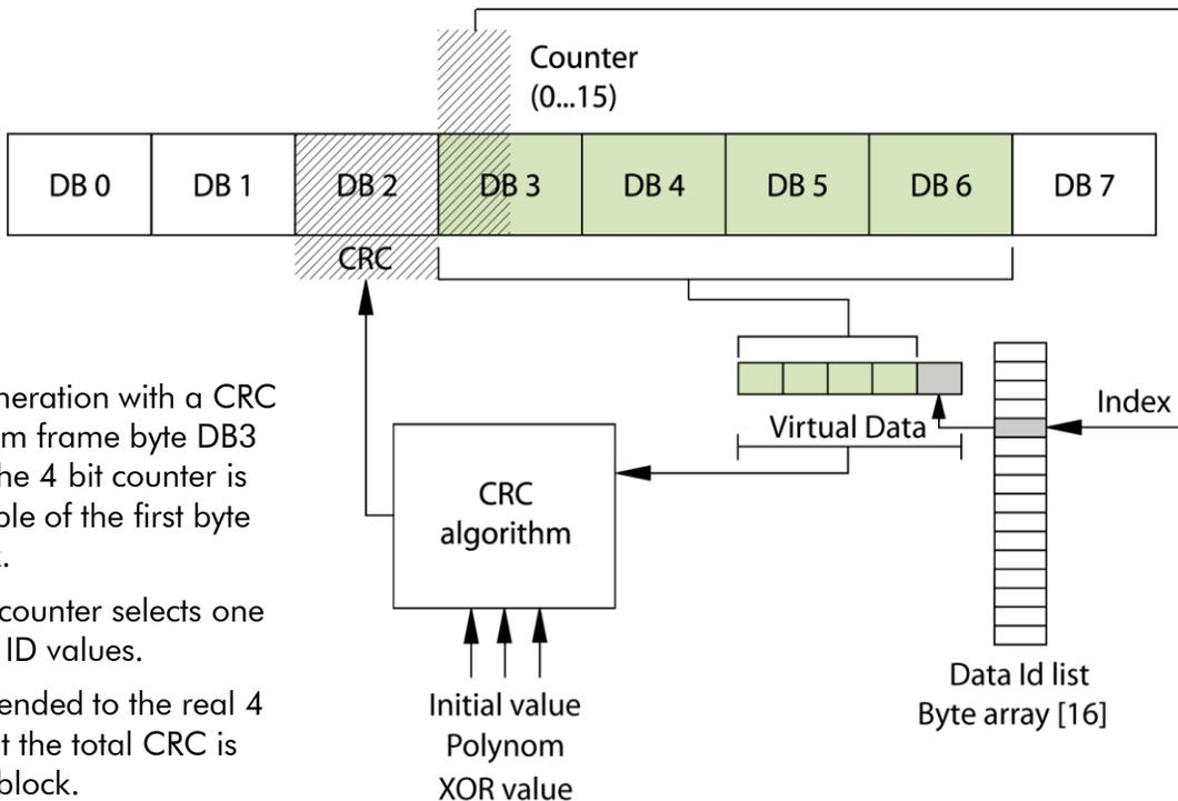
Example of a CRC generation with a CRC data block starting from frame byte DB3 to Autosar Profile 2. The 4 bit counter is located in the low nibble of the first byte of the CRC data block.
